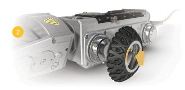
wheel attachment: align triangular lobes of hub with corresponding recesses on back side of wheel · push wheel firmly into place
