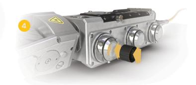
**hub detachment:** press removal tool into hub's o-ring groove  $\cdot$  unthread fastener · pull hub from axle
