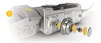
**hub attachment:** align key-ways and slide hub onto axle · slide o-ring onto screw  $\cdot$  apply a drop of Loc-tite to screw threads  $\cdot$  thread screw through hub into axle  $\cdot$  push hub cover snugly into place
