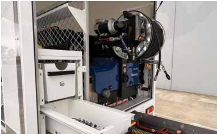
Picture of a Hino Hybrid truck fitted with the electric eCityJet Jetter by Rioned and iPek Rovion Camera system
