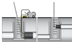
ALWAYS BLOCK PLUGS WHEN CONDUCTING AIR TESTS.
