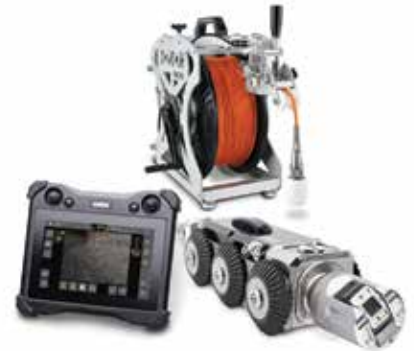
VC500 control with RM200 reel & RX95 crawler and PTC50 camera Standard Range - 200m portable system 100 - 300mm* *with extra-large wheel set
