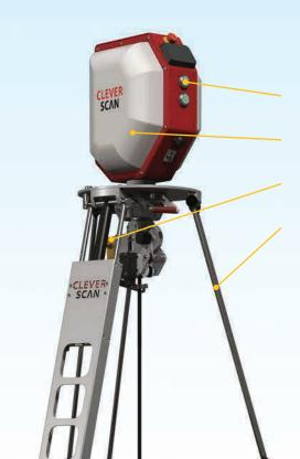
Fully automated system scans manholes with the press of a button.
